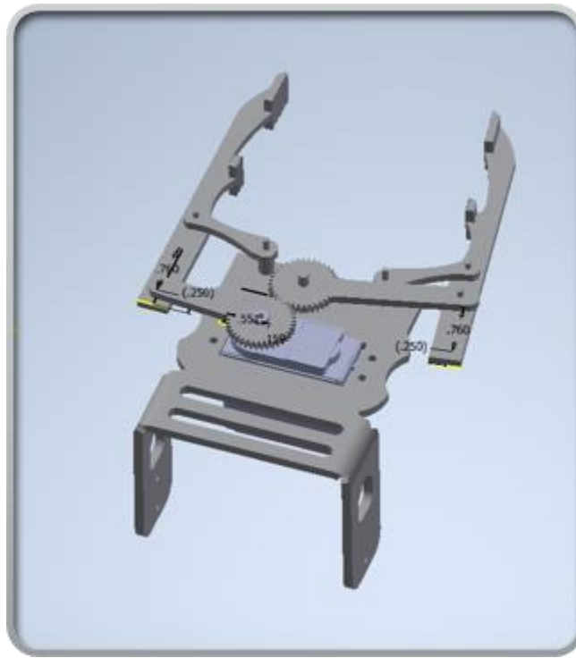
Figure 15: Claw Design (Assembled)
