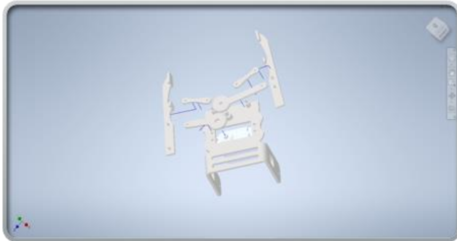
Figure 13: Claw Design (Exploded View)
